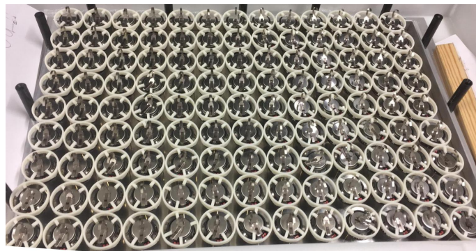
Figure 3.4: Several Kilobots improved by the designed 3D printed external structure. These were used in other projects and studies related to swarm robotics (no interest in springs connections).
