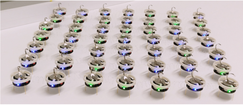
Figure 3.5: A 7x7 Kilobot Soft Robot composed of 49 modules connected by 84 light-weight springs. The LEDs show the battery level. The battery is considered discharged if the light is yellow or red.
