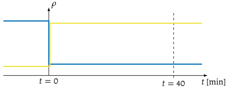
Figure 4.1: Colour concentration during the adaptation experiments. To study the ability of adaptation of the robot swarm, we assume that in the beginning of the experiments ( t = 0 minutes) the colour concentration instantaneously changes from higher concentration of blue to higher concentration of yellow. One experiment takes 40 minutes.
