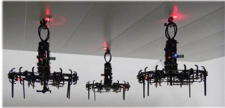
As reference models for the robots we consider the *eye-bot* robots, that have been developed in the Swarmanoid project (<http://www.swarmanoid.org>). Each robot is equipped with a video camera pointing to the floor, and has an infrared system for measuring the relative bearing and distance between two robots and for wireless communications.
