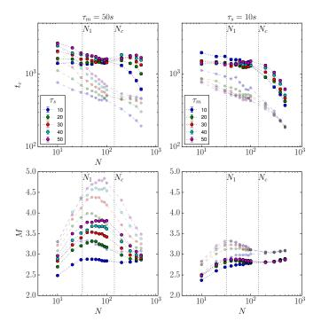
Fig. 4. Comparison between multiagent and robot simulations. Average values from multiagent simulations are shown with transparent colours, and serve as reference to appreciate the results from robotic simulations. Statistical error bars are not visible on the scale of the graphs. (Top) Convergence time  $t_c$ . (Bottom) Required memory *M*. (Left) Results for  $\tau_m = 50$ s, and varying  $\tau_s$ . (Right) Results for  $\tau_s = 10$ s, and varying  $\tau_m$ .
