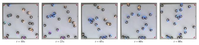
Fig. 5. Different shots of an experiment with 20 kilobots, with  $\tau_s = \tau_m = 2.5$  s (see also the supplementary video at http://ieeexplore.ieee.org). Robots lighting their LED have only one word in their inventory, while no color signal indicates more than one word or an empty inventory. Different words correspond to different colours.
