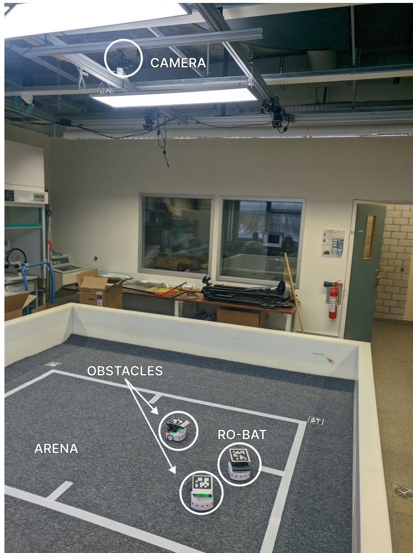
Figure 4.1: Setup used for the experiments in the lab where the arena is created by using white tape on the dark floor. I positioned additional tape on each side to allow the ro-bat to occupy also the middle part of the arena instead of moving only around the external parts.
