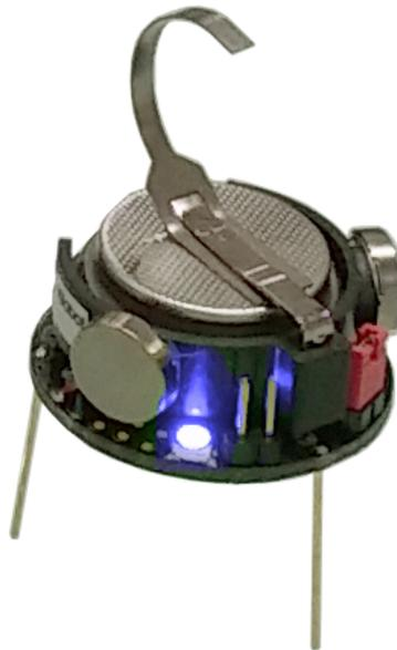
Fig. 3.3 A picture of the Kilobot robot
